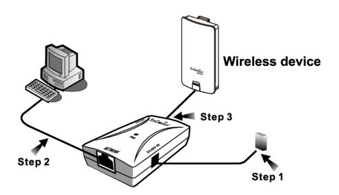
**Step1**: Plug the DC plug of AC/DC power adapter into a port of Inline Power Injection and the plug into a power outlet or power strip.
